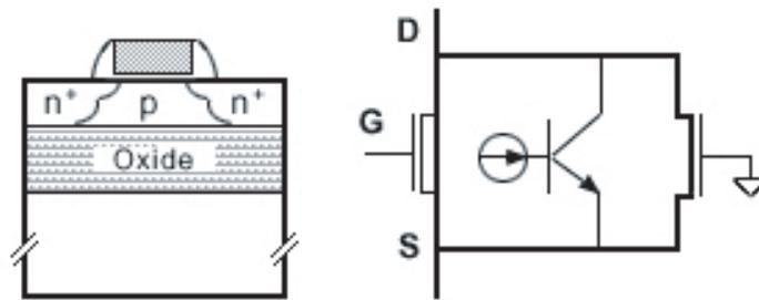
Schematic of nFET on SOI and equivalent devices.
