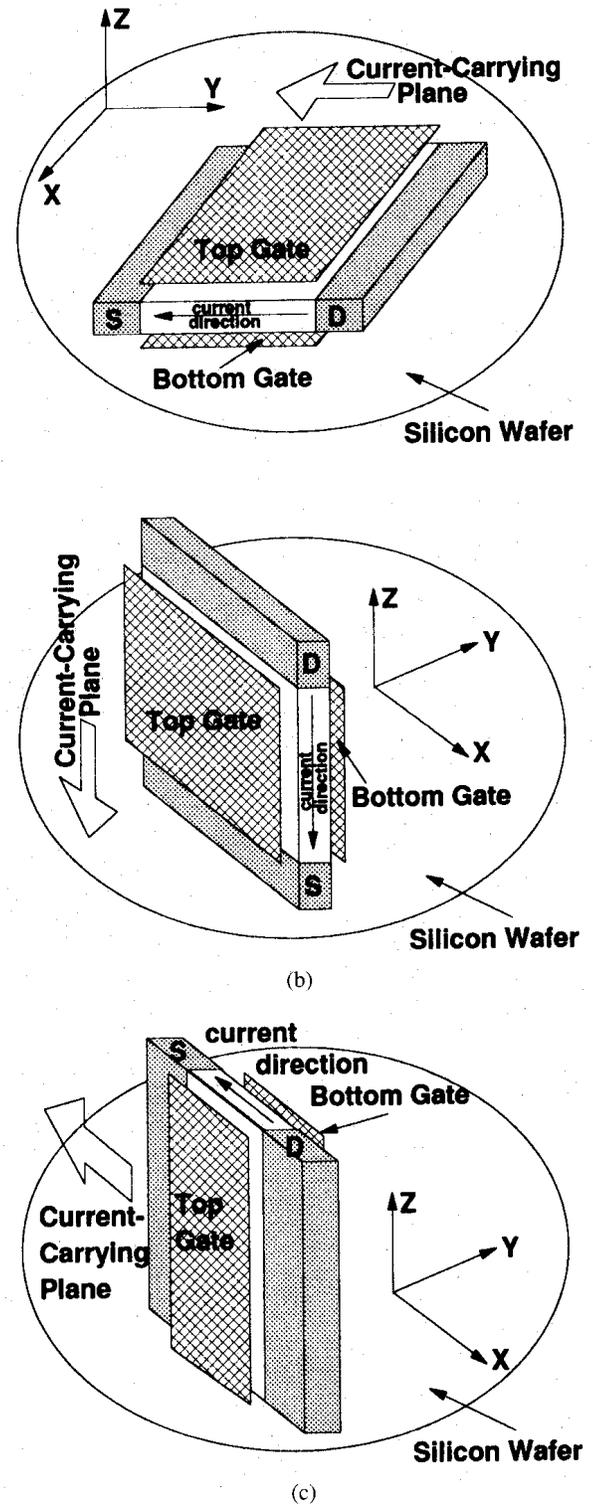
Fig. 29. Three possible orientations of a double-gate MOSFET on a silicon wafer. Examples of devices fabricated are: (a) Colinge et al. [54], Tanaka et al. [55], (b) Takato et al. [56], and (c) Hisamoto et al. [57].
