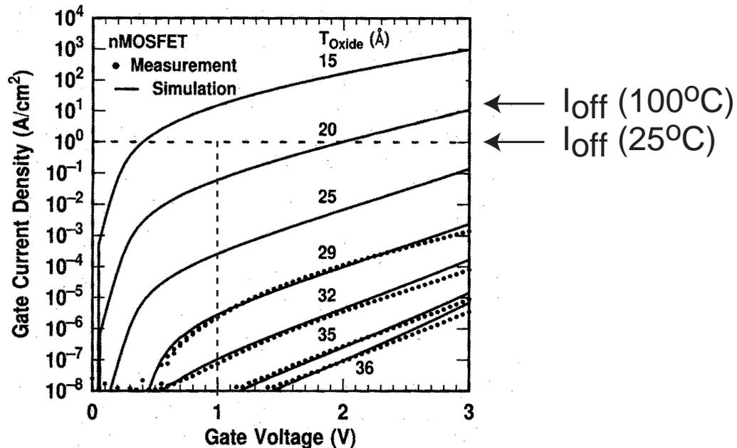
Fig. 2. Measured and simulated  $I_G$ - $V_G$  characteristics under inversion conditions of four nMOSFET's. The dotted line indicates the  $1 \text{ A/cm}^2$  limit for leakage current as discussed in the text.
