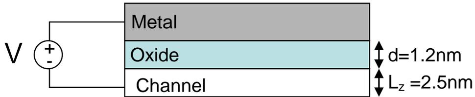
**Fig. 2.28.** A simple model of a modern transistor.
