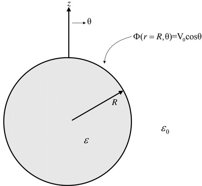
A dielectric sphere with permittivity  $\epsilon$  and radius  $R$  has a potential imposed at  $r = R$
