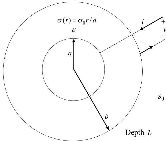
2. (30 points) Concentric cylindrical electrodes with respective radii  $a$  and  $b$  and depth  $L$  are surrounded by free space with permittivity  $\epsilon_0$  and encloses an ohmic material for  $a < r < b$  whose conductivity varies with radius as  $\sigma(r) = \sigma_0 r / a$  and has constant permittivity  $\epsilon$ . A voltage  $v$  is applied across the cylindrical electrodes. Neglect end effects at the top and bottom of the cylinder.
