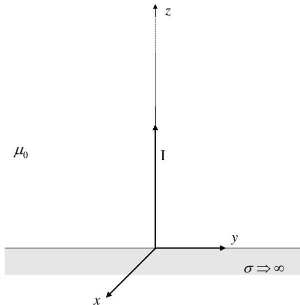
1. (30 points) A line current of semi-infinite length stands perpendicularly upon a perfectly conducting ground plane at  $z = 0$ .
