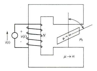
The inductance of the magnetic circuit varies with rotor angle  $\theta$  as
