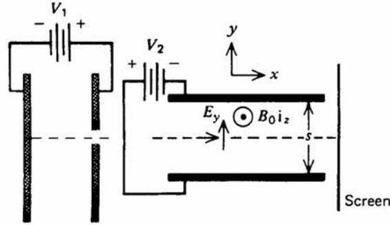
Figure 6: A diagram of a cathode-ray tube.
