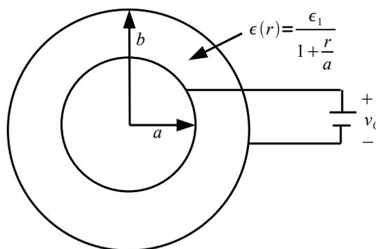
Figure 27: Concentric spherical electrodes enclose a dielectric with permittivity that varies with  $r$  with no volume charge in the dielectric (Image by MIT OpenCourseWare).
