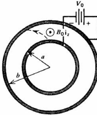
Figure 9: A diagram of two concentric conducting cylinders connected to a voltage source creating a magnetron.
