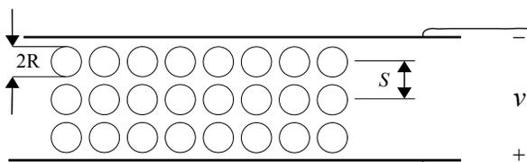
Figure 39: A diagram showing an artificial dielectric constructed of an array of conducting spheres (Image by MIT OpenCourseWare).
