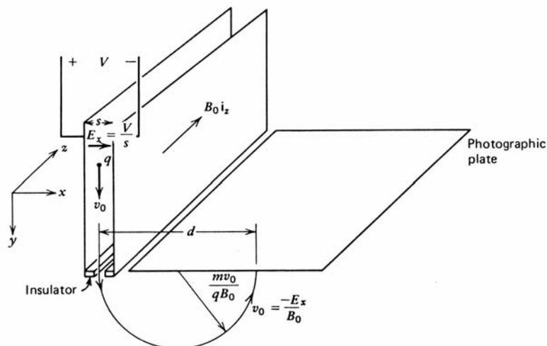
Figure 7: A diagram of a mass spectrograph.
