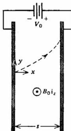
Figure 8: A diagram of two parallel plates connected to a power source creating a magnetron.
