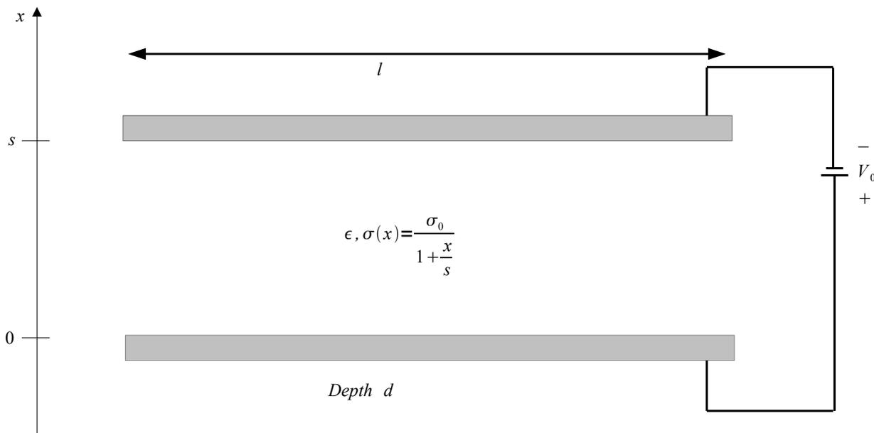
Figure 25: A diagram of parallel plate electrodes enclosing a lossy dielectric with  $x$  dependent conductivity (Image by MIT OpenCourseWare).
