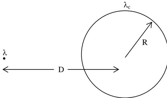
**(Hint:** Where can another image charge be placed with the cylinder remaining an equipotential surface?)
