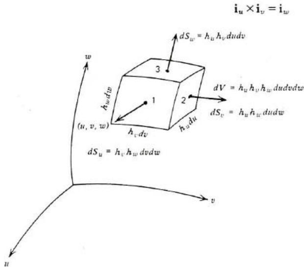
Since the incremental coordinate quantities  $du$ ,  $dv$ , and  $dw$  do not necessarily have units of length, the differential length elements must be multiplied by coefficients that generally are a function of  $u$ ,  $v$ , and  $w$ :
