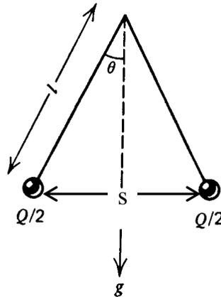
A total charge  $Q$  is deposited on the two identical balls of the electroscope when they are touching. The balls then repel each other and the string is at an angle  $\theta$  from the normal which obeys a relation of the form
