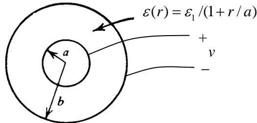
Concentric spherical electrodes with respective radii  $a$  and  $b$  enclose a material whose permittivity varies with radius as  $\epsilon(r) = \epsilon_1 / (1 + r/a)$ . A voltage  $v$  is applied across the spherical electrodes. There is no volume charge in the dielectric.
