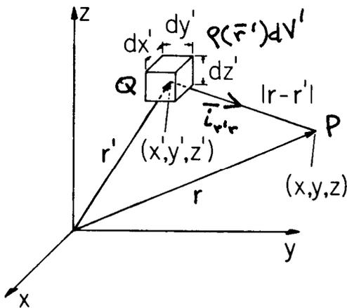
**Figure 4.5.1** An elementary volume of charge at  $\mathbf{r}'$  gives rise to a potential at the observer position  $\mathbf{r}$ .
