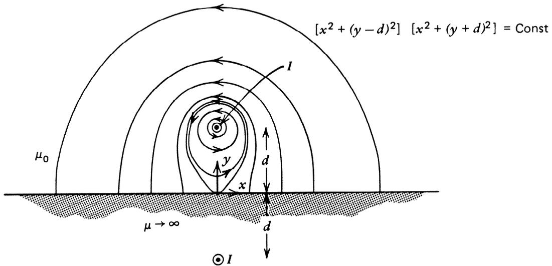
A line current  $I$  of infinite extent in the  $z$  direction is at a distance  $d$  above an infinitely permeable material as shown above.
