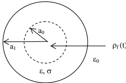
What is the time dependence of the electric field everywhere and the free surface charge density at  $r=a_1$  as a function of time? At time  $t=0$  the surface charge at  $r=a_1$  is zero.
