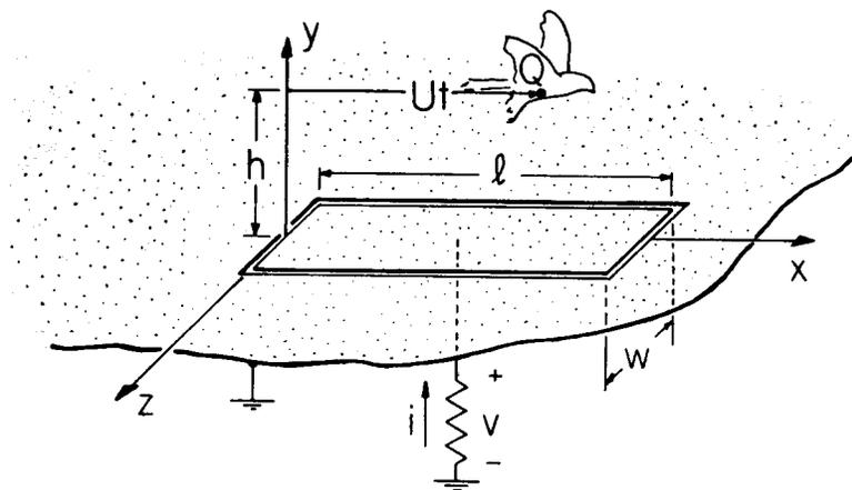
"Bird on Powerline" diagram from: *Electromagnetic Fields and Energy* by Hermann A. Haus and James R. Melcher.
