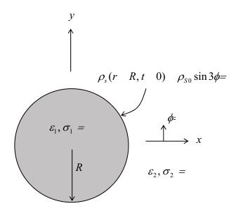
A cylinder of radius R and infinite extent in the z direction with dielectric permittivity  $\varepsilon_1$  and ohmic conductivity  $\sigma_1$  is placed within a medium of infinite extent that has permittivity  $\varepsilon_2$  and ohmic conductivity  $\sigma_2$ . At time t=0 the free surface charge density on the r=R interface is  $\rho_s(r-R,t-0)-\rho_{s0}\sin 3\phi$ .
