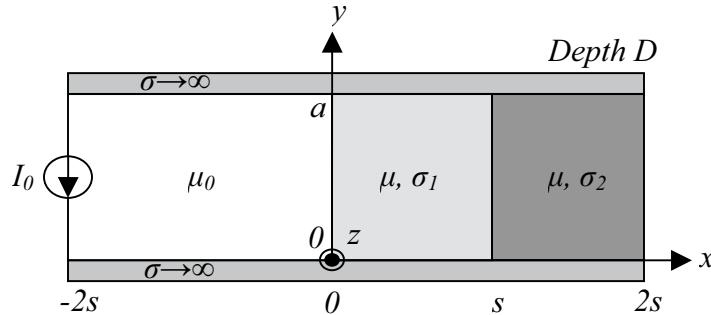
A DC current source  $I_0$  is connected to two perfectly conducting planes with spacing  $a$  and length  $4s$ . Two conducting blocks, each with the same width  $s$  and the same magnetic permeability  $\mu$ , have different respective ohmic conductivities  $\sigma_1$  and  $\sigma_2$ , and are placed side by side in the region  $0 < x < 2s$  as shown in the above figure.
