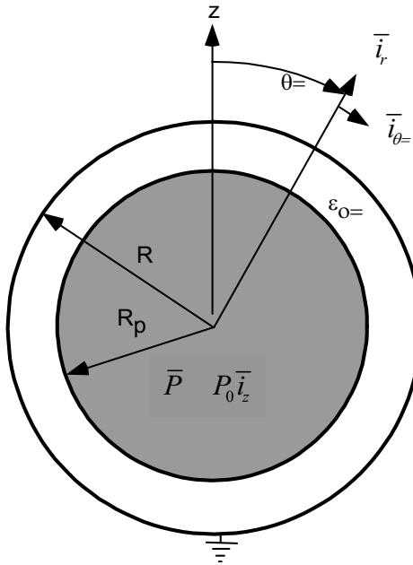
A sphere with radius  $R_p$  is comprised of permanently polarized material uniformly polarized in the  $z$  direction,  $P_0 \vec{i}_z$ . The sphere is placed concentric with a second, grounded, perfectly-conducting sphere of radius  $R$  as shown in the cross-sectional drawing in the figure above. The region  $R_p < r < R$  is filled with free space with dielectric permittivity  $\epsilon_0$ . There is no free surface charge on the  $r=R_p$  interface.
