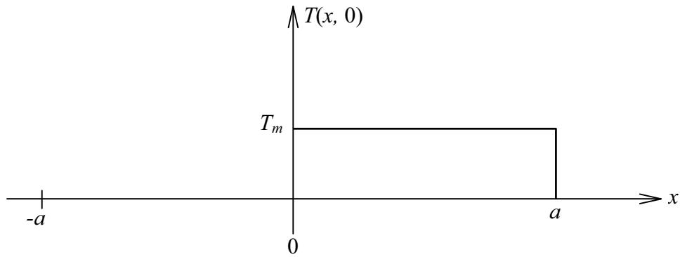
A thin elastic rod of length  $2a$  is placed on the  $x$  axis and extends from  $-a < x < a$ . The initial velocity and stress distributions at  $t=0$  are:
