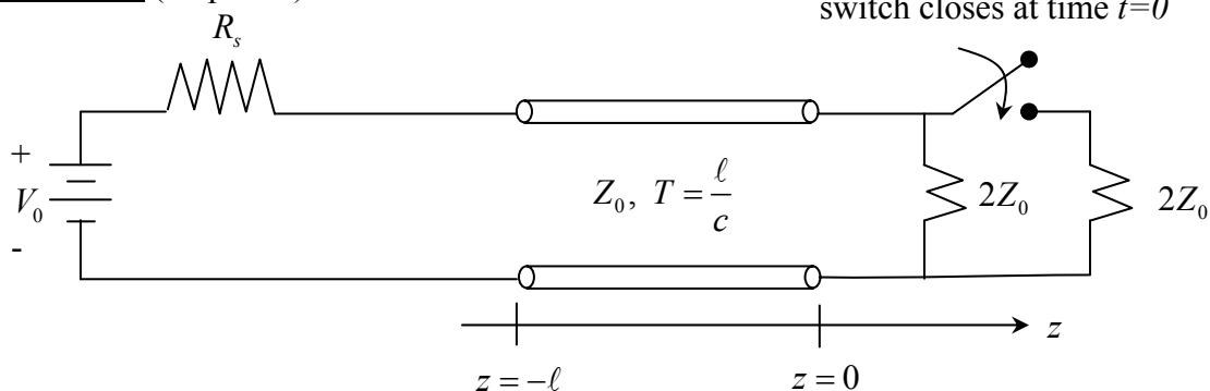
A transmission line with characteristic impedance  $Z_0$ , length  $l$  and wave speed  $c$  has a load at  $z=0$  of  $2Z_0$  when the switch is open, and a load of  $Z_0$  when the switch is closed. At  $z=-l$ , the transmission line is connected to a DC voltage  $V_0$  and series source resistance  $R_s$ .
