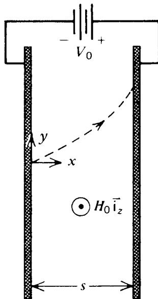
A magnetron is essentially a parallel plate capacitor stressed by constant voltage  $V_o$  where electrons of charge  $-e$  are emitted at  $x=0, y=0$  with zero initial velocity. A transverse magnetic field  $H_o \vec{i}_z$  is applied. Neglect the electric and magnetic fields due to the electrons in comparison to the applied field.
