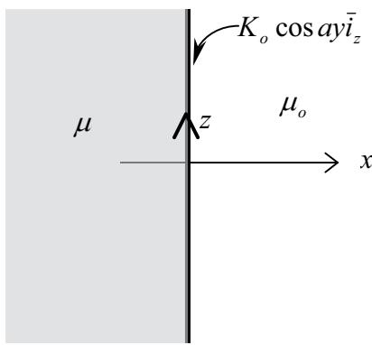
A current sheet  $K_o \cos(ay) \bar{i}_z$  is placed at  $x=0$  at the interface between a magnetic material with permeability  $\mu$  and free space. Because there are no volume currents for  $x \neq 0$ , a scalar magnetic potential  $\psi$  can be defined such that
