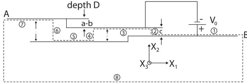
Figure 2: Diagram of surfaces (1)-(8) used to find force on the lower electrode using the Maxwell Stress Tensor. (Image by MIT OpenCourseWare.)
