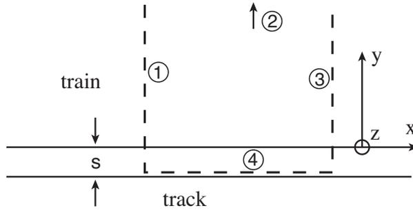
Figure 5: Diagram of the Maxwell Stress Tensor surface to find the levitation force on a train. (Image by MIT OpenCourseWare.)
