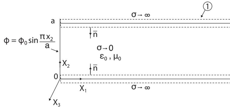
Figure 3: Diagram of grounded electrodes and distributed electric potential source at  $x_1 = 0$ . (Image by MIT OpenCourseWare.)
