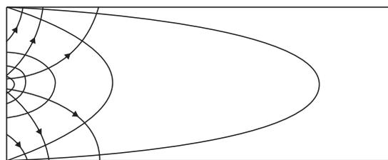
Figure 4: Sketch of the  $\vec{E}$  field and equipotential lines. (Image by MIT OpenCourseWare.)
