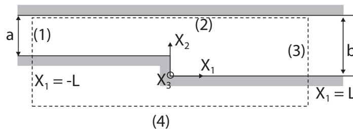
Figure 1: Diagram of surfaces (1), (2), (3), and (4) to evaluate the force on the lower plate using the Maxwell Stress Tensor. (Image by MIT OpenCourseWare.)
