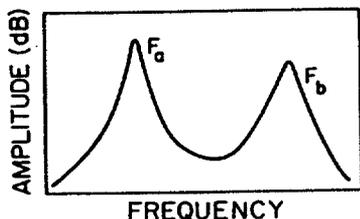
Figure 4.32 Schematization of the spectrum envelope of a two-formant sound used in the matching experiments of Chistovich and Lublinskaya (1979). The frequency spacing  $F_b - F_a$  and the relative amplitudes of the spectral prominences were manipulated.
