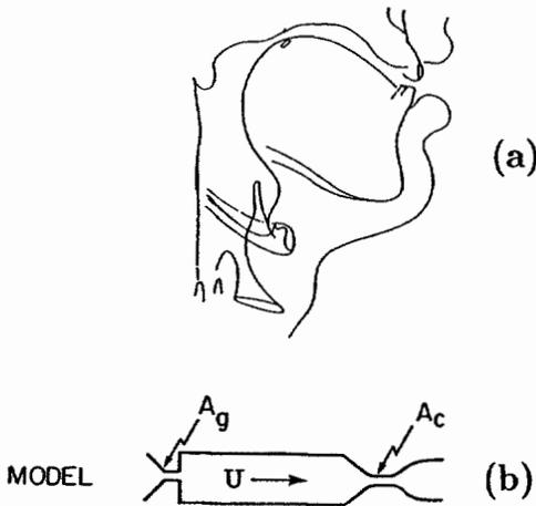
Figure 8.50 (a) Midsagittal section of vocal tract for vowel /i/, showing constriction in the palatal region. (From Perkell, 1969.) (b) Schematization of the airway with two constrictions—one at the glottis, with cross-sectional area  $A_g$ , and the other in the supraglottal airway, with cross-sectional area  $A_c$ .
