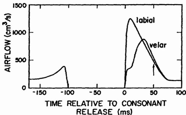
Figure 8.60 Calculated values of airflow versus time for intervocalic voiceless aspirated stop consonants, corresponding to the time variation of glottal and supraglottal areas given in figure 8.58. Calculations are based on the equivalent circuit in figure 8.59, with a subglottal pressure of 8 cm  $H_2O$ . Element values for  $C_w$  and  $R_w$  are given in the legend for figure 7.4. The estimated time of onset of vocal fold vibration is indicated by the arrow at 50 ms.
