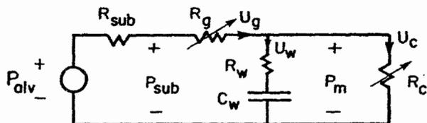
Figure 8.59 Equivalent circuit used to calculate the flows and pressures at the release of a voiceless aspirated stop consonant. Values of the elements are discussed in the text and in the legend to figure 7.4.  $R_{sub} = 1.5$  acoustic ohms.
