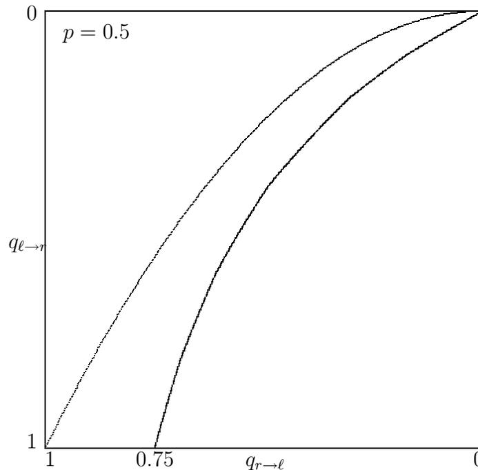
Figure 4. EXIT chart for iterative decoding of a rate- $\frac{1}{3}$  RA code on a BEC with  $p = 0.5$ .
