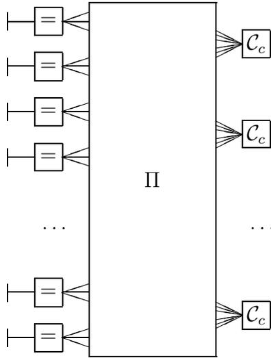
Figure 5. Normal graph realization of  $\mathcal{C}$ , with left repetition constraints of degree  $d_\lambda$  and right constraint codes  $\mathcal{C}_c$  of degree  $d_\rho$ .
