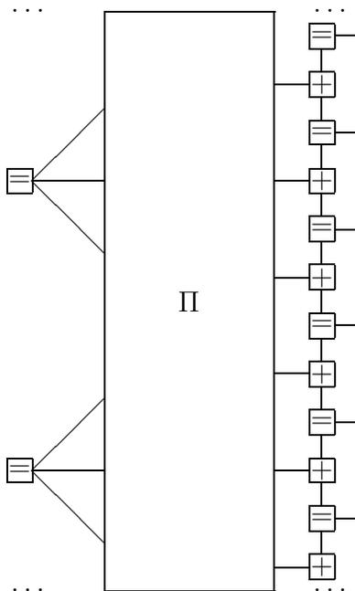
Figure 3. Normal graph of rate- $\frac{1}{3}$  RA code.
