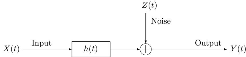
Figure 1.5: Linear Gaussian channel model.
