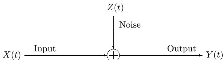
Figure 1.4: An additive white Gaussian noise (AWGN) channel.
