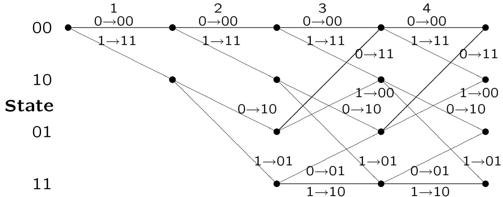
**Viterbi decoding: At each epoch, decode conditional on each possible assumed state.**
