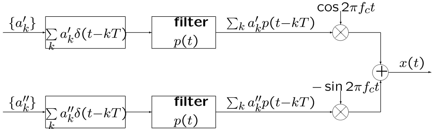
**Demodulate by multiplying  $x(t)$  by both cosine and sign. Then filter out components around  $2f_c$ .**
