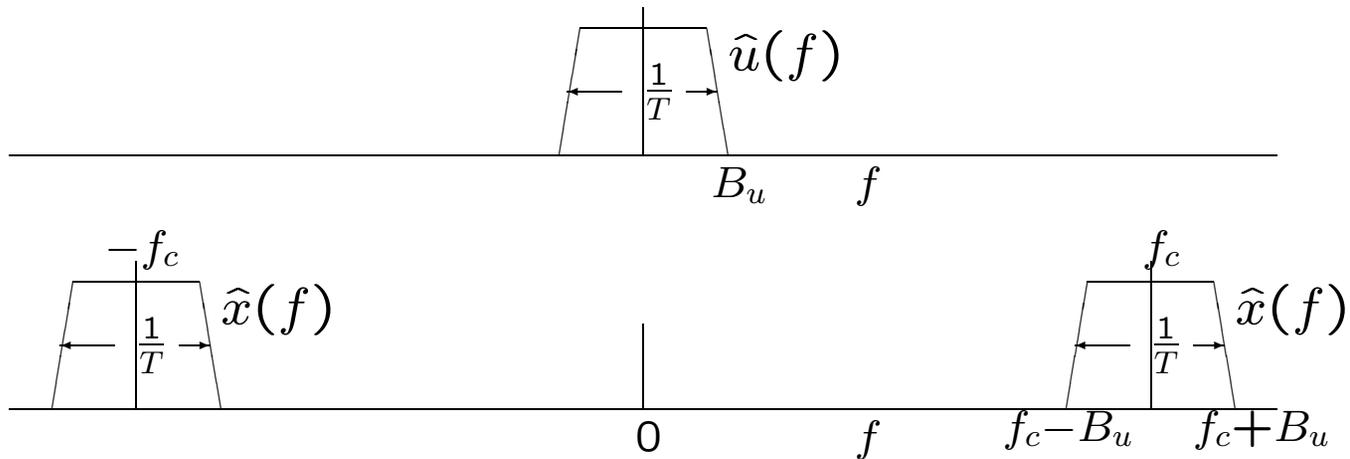
**The bandwidth  $B$  is  $2B_u$ . The bandwidth is always the range of positive frequencies used.**
