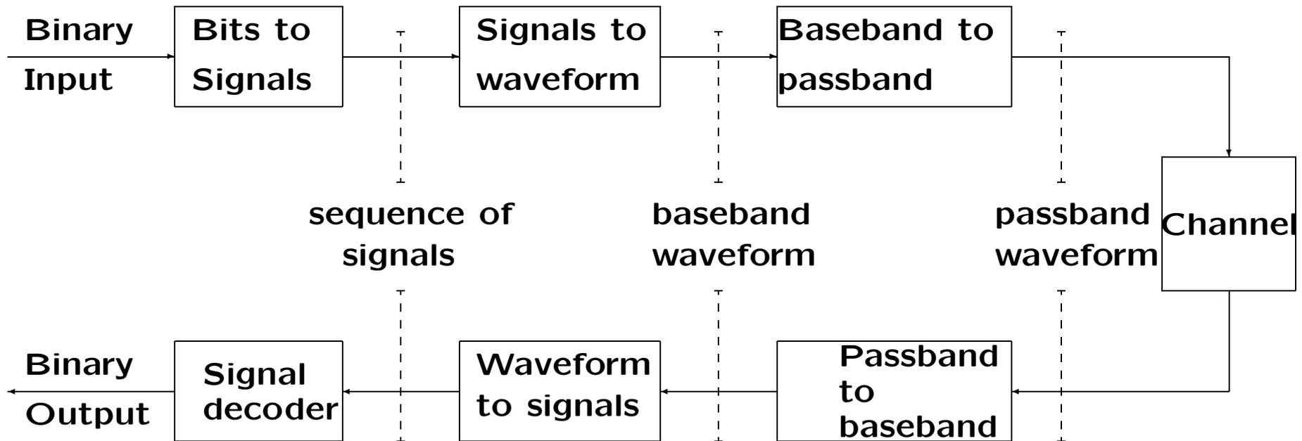
For now we focus on the baseband transmitted waveform  $u(t)$  and the received baseband waveform  $v(t)$ .
