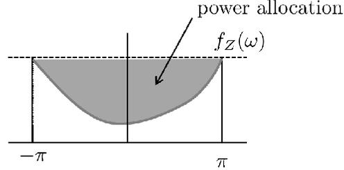
waterfilling across spectrum for stationary ACGN channel
