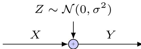
**Definition 17.5** (AWGN). The additive Gaussian noise (AWGN) channel is a stationary memoryless additive-noise channel with separable cost constraint:  $\mathcal{A} = \mathcal{B} = \mathbb{R}$ ,  $c(x) = x^2$ ,  $P_{Y|X}$  is given by  $Y = X + Z$ , where  $Z \sim \mathcal{N}(0, \sigma^2) \perp X$ , and average power constraint  $\mathbb{E}X^2 \leq P$ .
