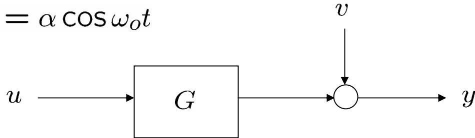
$$y(t) = \alpha |G(e^{i\omega_o})| \cos(\omega_o t + \phi) + v(t) + \text{transients}$$
