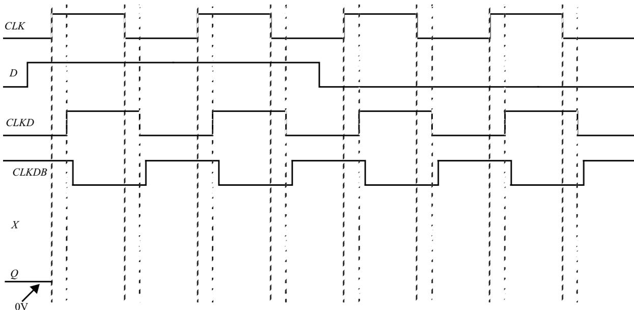
b) What is the set-up time for this circuit if glitches on the output  $Q$  are acceptable? Explain.
