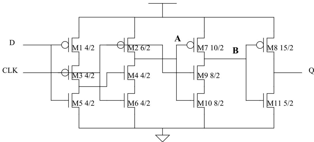
Simulate the circuit in HSPICE. The sizes of the devices are given in terms of lamda. Make sure you initialize node B and that you use stimuli given below.
