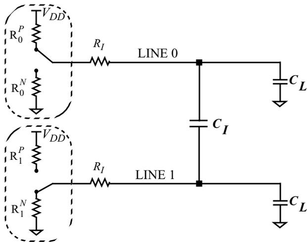
(a) Assume that the initial voltage on line  $i$  (where  $i = 0$  or  $1$ ) is  $V_i^{OLD}$  and the final value after all the transients have settled is  $V_i^{NEW}$ .  $V_i^{OLD}, V_i^{NEW} \in \{0, V_{DD}\}$ . Derive an expression for the energy drawn from  $V_{DD}$  through *driver 0* for an arbitrary transition of the two bit bus.
