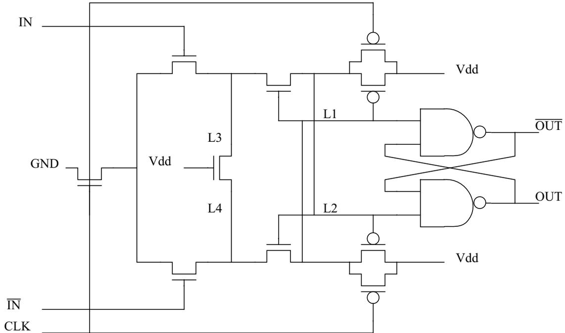
The flip-flop shown in the above figure is used in the StrongARM microprocessor developed by Digital Equipment Corporation for the Portable Electronic Device (PED) market. Note that it is fully differential. The following questions will help you understand the operation of this flip-flop. No calculations are necessary for this problem.
