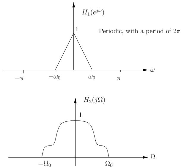
Figure 2-2: Frequency responses of discrete-time LTI filter  $H_1$  and continuous-time LTI filter  $H_2$ .
