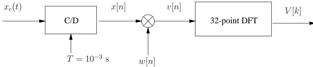
Figure 6-1: Spectral analysis system.
