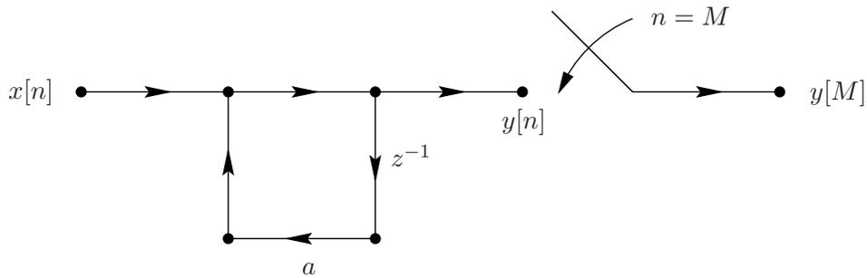
Figure 9-1: System for calculating  $y[M]$  from  $x[n]$ .
