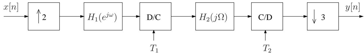
Figure 2-1: System for calculating  $y[n]$  from  $x[n]$ .
