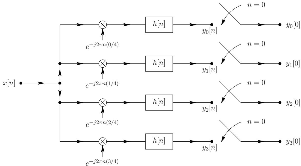
Figure 8-1: Filter bank network.
