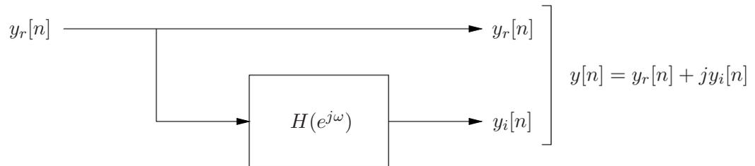
Figure 1-1: System for obtaining  $y[n]$  from  $y_r[n]$ .
