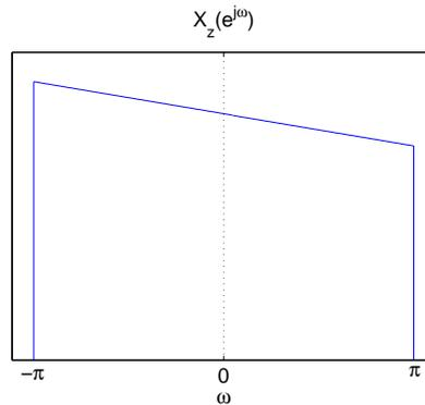
Taking the DFT of  $x_z[n]$  gives us  $N$  samples of  $X_z(e^{j\omega})$  spaced  $\frac{2\pi}{N}$  apart in frequency. By comparing Figure P10.44-2 with the sketch of  $X_z(e^{j\omega})$  above, we see that these samples are the desired samples of  $X(e^{j\omega})$  spaced by  $\frac{2\Delta\omega}{N}$  from  $\omega_c - \Delta\omega$  to  $\omega_c + \Delta\omega$ .
