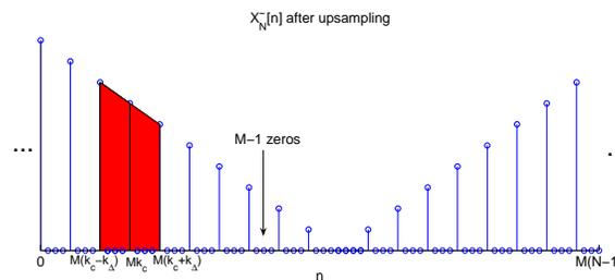
Filtering by  $h[n]$  interpolates between the non-zero samples. We assume that  $h[n]$  is an ideal zero-phase filter in sketching  $\tilde{X}_{MN}[n]$ . The interpolated points are marked with an  $\times$ .
