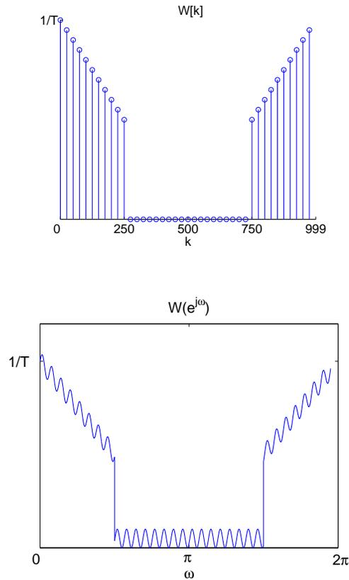
We obtain  $y[n]$  by compressing  $w[n]$  by 2 and padding the result with 500 zeroes. The DTFT  $Y(e^{j\omega})$  is given by
