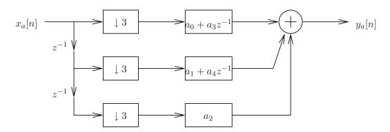
This is efficient because the filtering is done at the lowest possible sampling rate.
