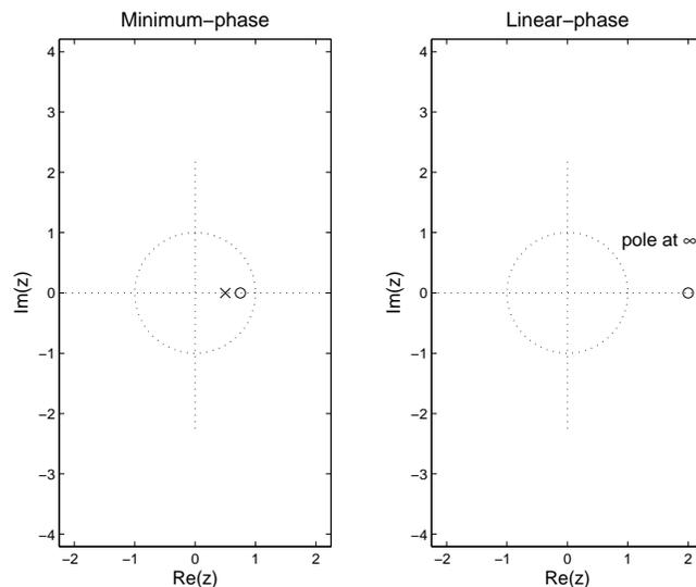
Next, we need to modify the first stage because we need to make sure that the linear-phase FIR system really is linear-phase FIR, so add a zero at  $z = 1/2$ . Since the system has to have the same number of zeros and poles, we also need to add a pole. For an FIR system, the pole must be at  $z = 0$  or at  $z = \infty$ . We choose to add the pole at  $z = 0$  because we will have to cancel the pole by a zero in the minimum-phase system.
