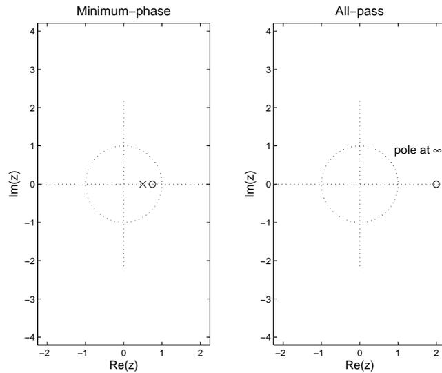
Next, we need to modify the first stage because we need to make sure that the all-pass system really is all-pass, so add a pole at  $z = 1/2$  and a zero at  $z = 0$ .
