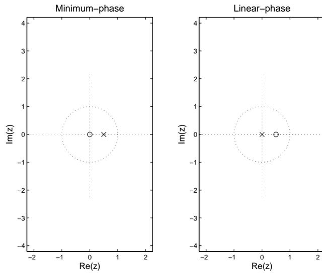
Combining these, the minimum-phase system and FIR linear-phase systems are as shown below.
