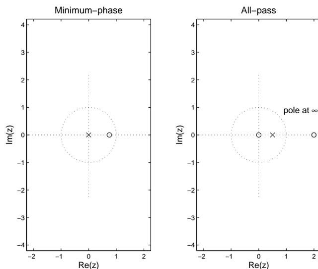
In the minimum-phase system, the pole at  $z = 1/2$  from the first stage has been cancelled by the zero added in the second stage. Another way to look at that is that for this particular system, we started with an all-pass pair (a pole at  $z = 1/2$  and a zero at  $z = 2$ , so we could have put these into the all-pass system initially.
