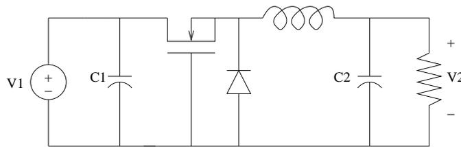
Figure 5.4: Buck (down) Converter
