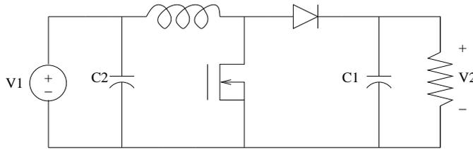
Figure 5.7: Boost (up) Converter Drawn Left to Right
