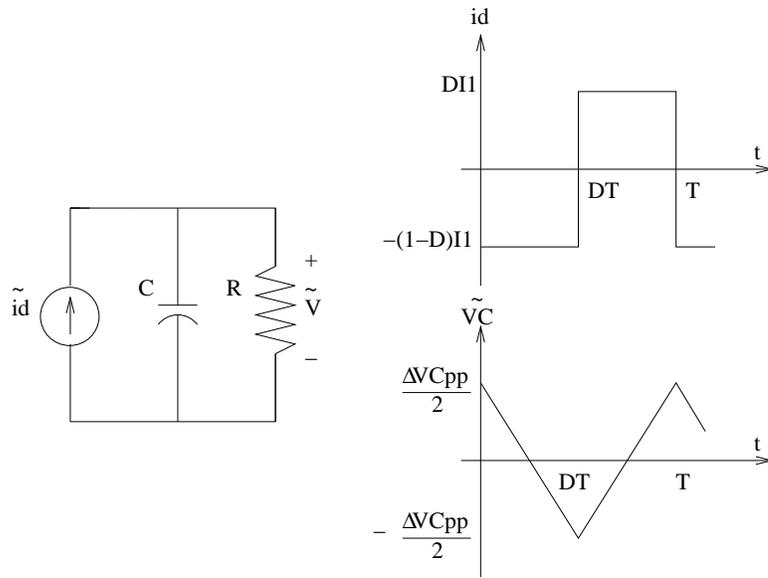
Figure 5.24: Ripple Model with Capacitor
