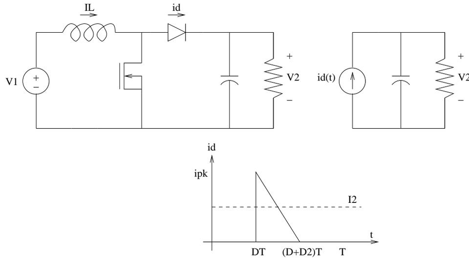
Figure 5.31: DCM Operation Model
