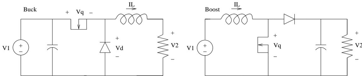
Figure 5.21: Direct Converters (neglecting ripple)
