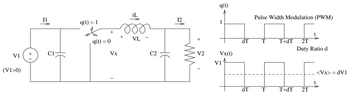
Figure 5.3: DC/DC Converter
