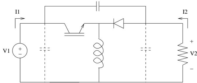
Figure 5.16: “Buck/Boost” or “up/down” converter
