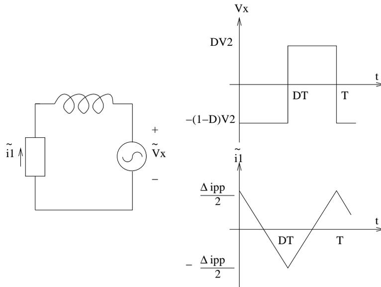
Figure 5.26: Ripple Model with Inductor
