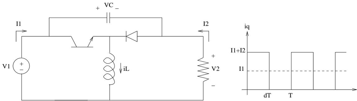
Figure 5.20: Indirect Converters (neglecting ripple)
