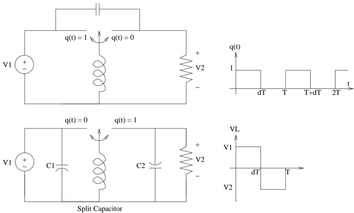
Figure 5.15: Indirect DC/DC Converter
