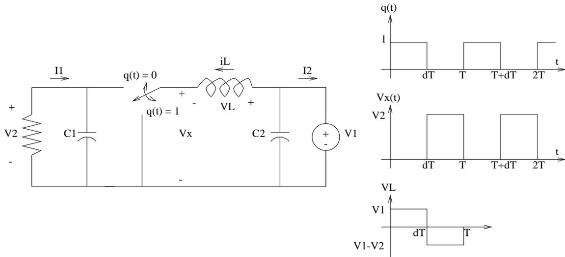
Figure 5.5: Change the Location of Source and Load
