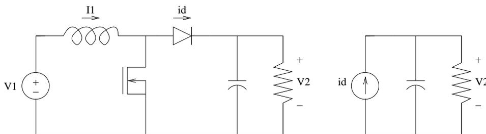
Figure 5.22: Boost Converter Ripple
