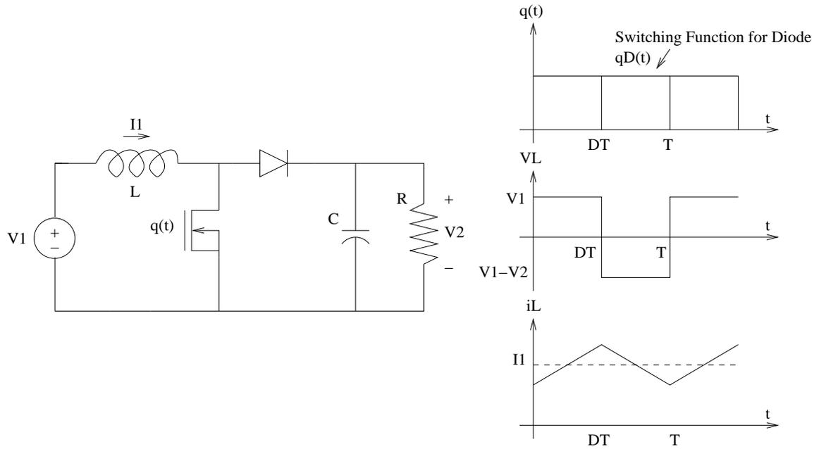
Figure 5.28: Boost Converter Waveforms
