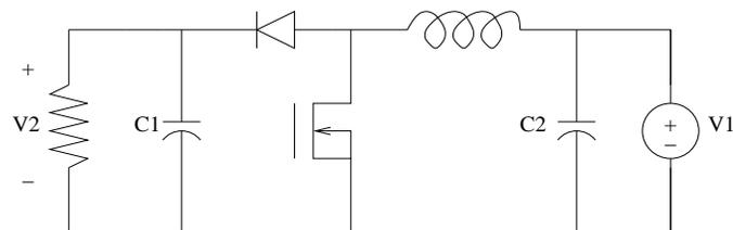
Figure 5.6: Boost (up) Converter
