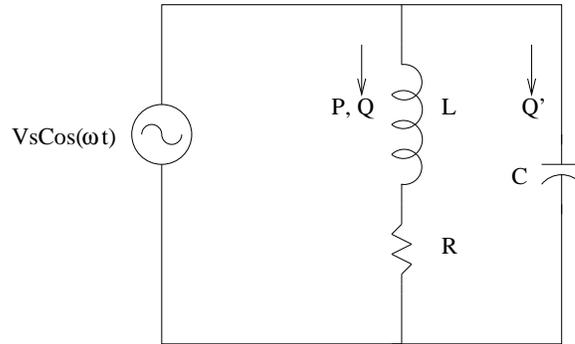
Figure 3.8: Parallel Capacitor
