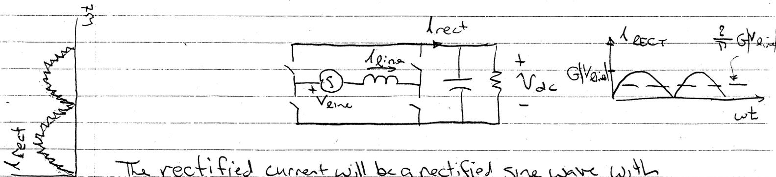
The rectified current will be a rectified sine wave with peak magnitude  $G V_{line}$  and average value  $\frac{2}{\pi} G V_{line}$
