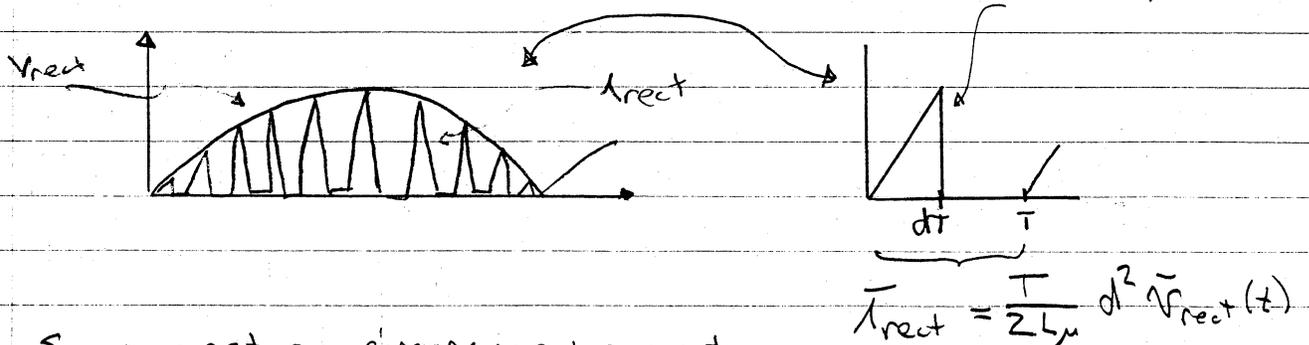
So we get an average input current proportional to the input voltage and the square of the duty ratio.
