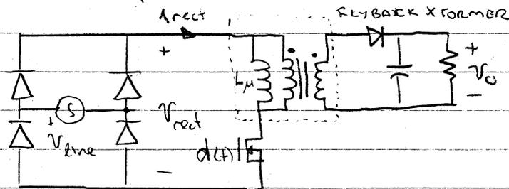
$$I_{pk} = \frac{V_{rect}}{L_{\mu}} dT$$
