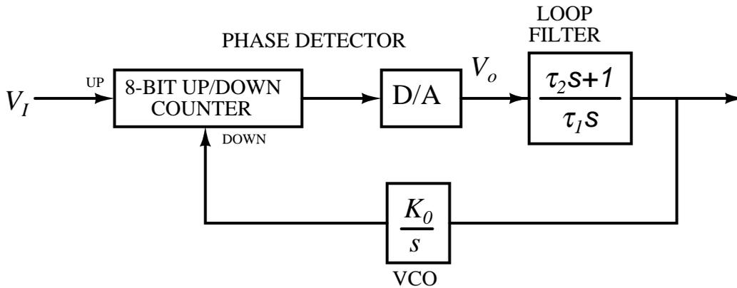
Figure 6.3: Alternative Digital Phase Detector
