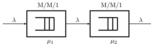
Figure 6.13: A tandem queueing system. Assuming that  $\lambda > \mu_1$  and  $\lambda > \mu_2$ , the departures from each queue are Poisson of rate  $\lambda$ .
