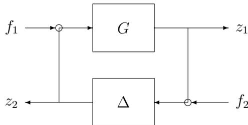
Figure 13.1: setup for the Small Gain Theorem
