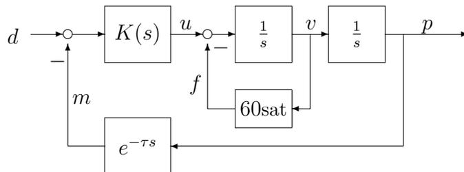
Figure 13.6: Example: a servo with friction
