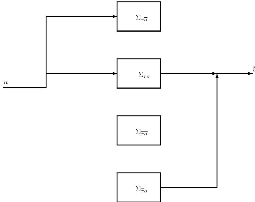
Figure 25.1: Kalman Decomposition of a State Space Model.
