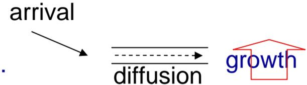
1)  $R > 1 \Rightarrow$  Non-equilibrium, fast growth, many misaligned islands form, leading to defective (high-surface-en), polycrystalline film, columnar grains, This 3-D growth is “*Volmer-Weber*” mode; Can  $\Rightarrow$  amorphous film.
