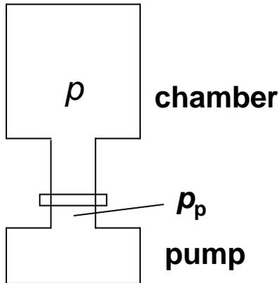
$$Q = C \left( \frac{Q}{S^{eff}} - \frac{Q}{S_p} \right) \Rightarrow S^{eff} = \frac{CS_p}{C + S_p} = \frac{1}{\frac{1}{C} + \frac{1}{S_p}}$$
