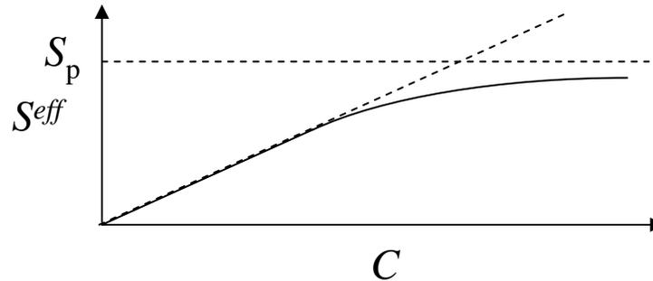
**Effective pump speed,  $S^{eff}$ , never exceeds conductance of worst component or pump speed,  $S_p$ .**
