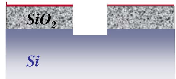
**How thick is 0.035  $\mu\text{m}$  mask after etch?**
