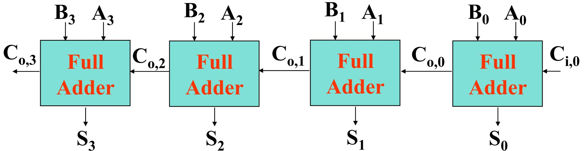
Worst case propagation delay linear with the number of bits
