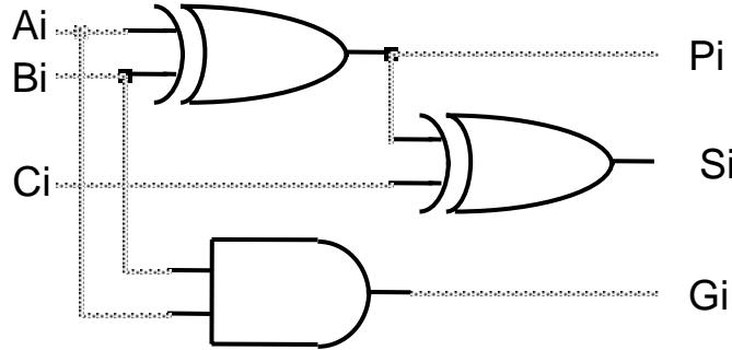
Adder with propagate and generate outputs
