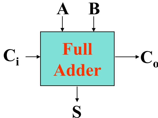
$$\begin{aligned} S &= A \oplus B \oplus C_i \\ &= A\bar{B}\bar{C}_i + \bar{A}BC_i + \bar{A}\bar{B}C_i + ABC_i \end{aligned}$$
