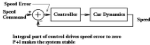
By measuring actual speed and feeding that back to the PI controller, we can drive speed error (exponentially) to zero.
