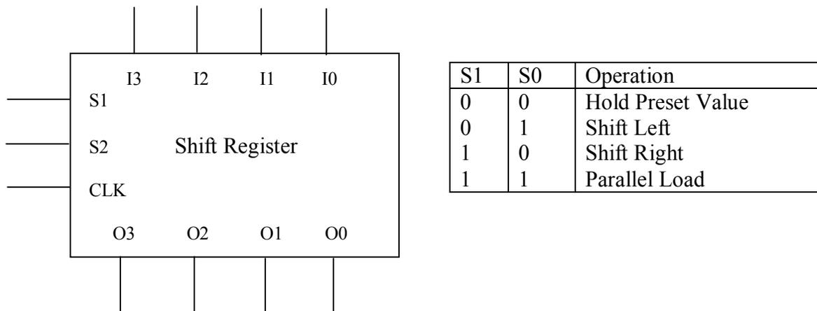
The circuit shown above is a 4-bit bi-directional circular shift register with parallel load. The adjacent truth table indicates the operation state based upon the two select lines. The inputs are labeled I3, I2, I1, and I0. The outputs are labeled O3, O2, O1, and O0. This device is a circular shift register. This means that when shifting left, bit 3 is shifted onto bit 0, and when shifting right bit 0 is shifted onto bit 3.
