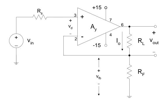
SERIES-SERIES FEEDBACK [NON-INVERTING AMPLIFIER, FLOATING LOAD, HIGH OUTPUT IMPEDANCE]
