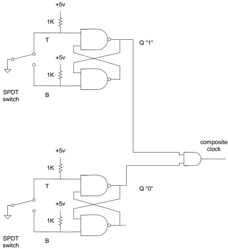
Verify with an oscilloscope that the debounce circuits function properly and a composite clock is generated.
