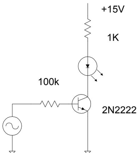
Turn on function generator and using a ramp signal try to get a pulsing light. Set the frequency low enough so that your eyes can see the pulse. You will also need to adjust the amplitude.
