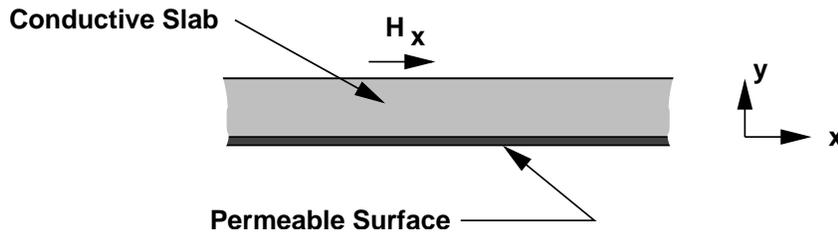
Figure 7: Axial View of Magnetic Field Problem
