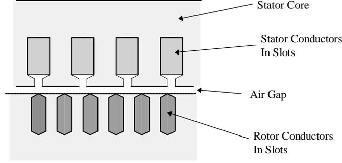
Figure 4: Windings in Slots
