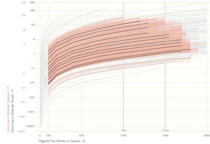
— Total core loss curves for this material, 50 through 2000 hertz
