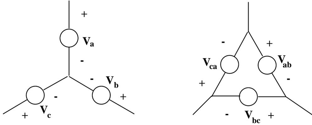
Figure 9: *Wye* And *Delta* Connected Voltage Sources
