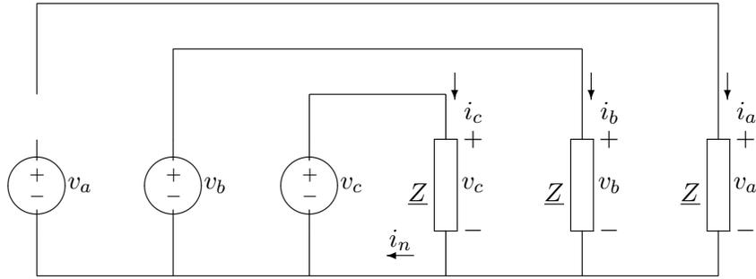
Figure 6: Three- Phase Source Connected To Balanced Load
