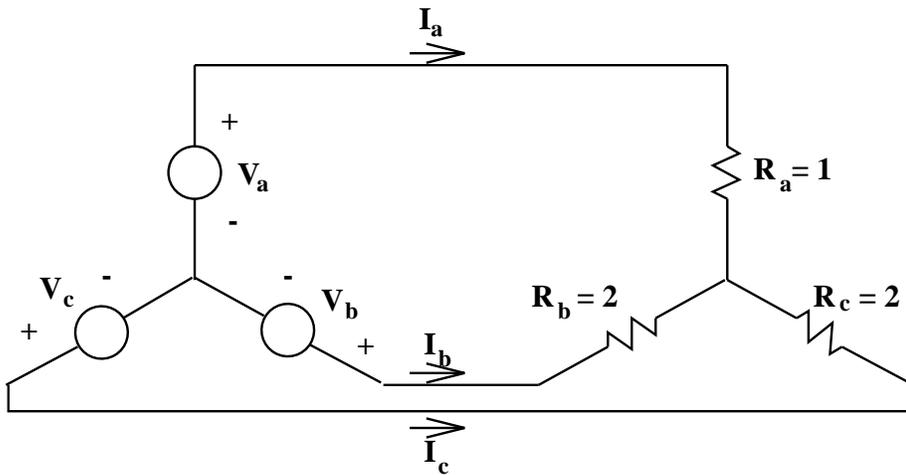
Figure 11: Unbalanced Load
