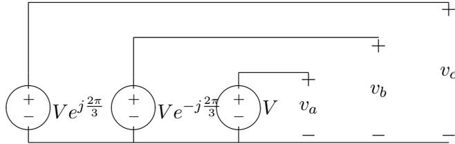
Figure 3: Three- Phase Voltage Source
