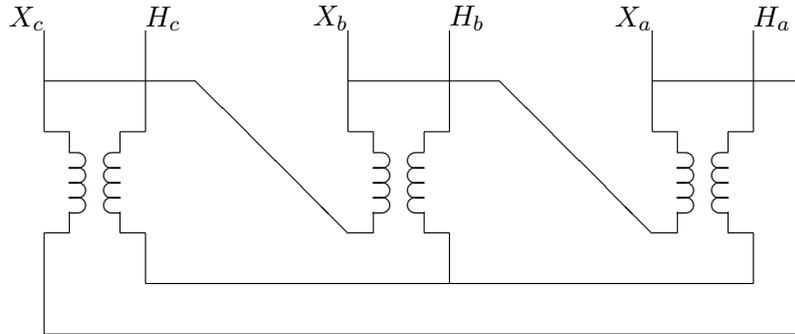
Figure 16: *Delta-Wye* Transformer Connection
