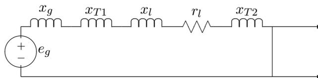
Figure 25: Impedance Diagram For Fault Example
