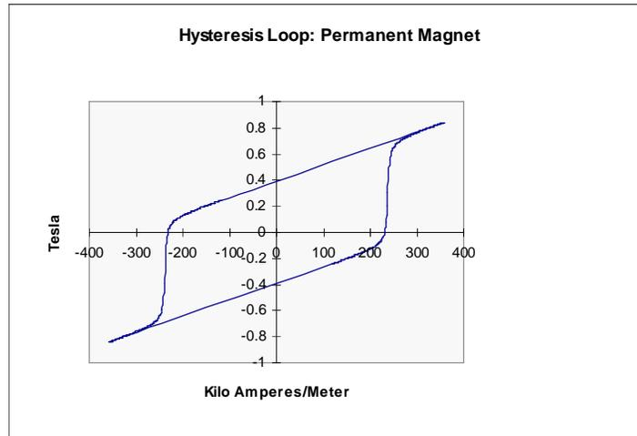
Figure 11: Hysteresis Loop Of Ceramic Permanent Magnet
