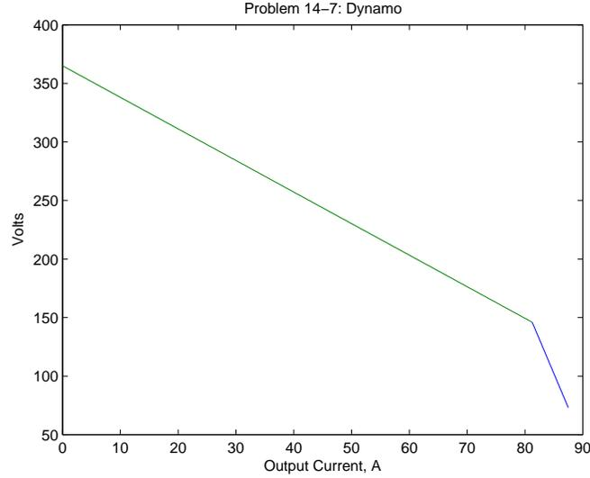
Figure 5: Voltage vs. Load Current
