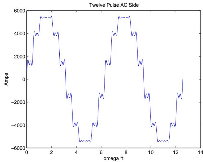
Figure 2: Reconstructed AC Waveform: Twelve Pulse
