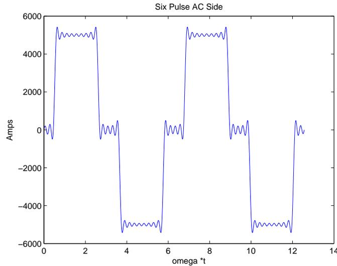
Figure 1: Reconstruction of Six Pulse Waveform, harmonics to order 25
