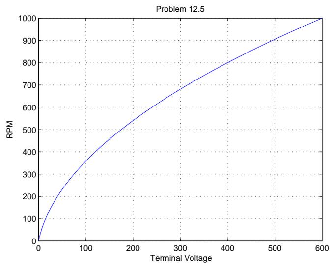
Figure 3: Speed vs. Voltage for Series Motor
