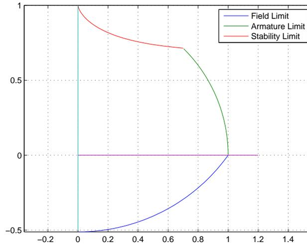
Figure 7: Capability Curve for Salient Pole Machine (per-unit)
