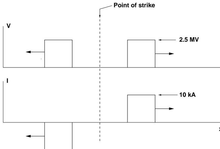
Figure 1: Pulses at about 40 microseconds
