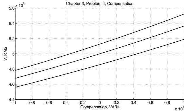
Figure 4: Receiving End Voltage
