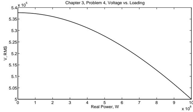
Figure 3: Receiving End Voltage
