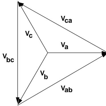
Figure 6: Three-Phase Voltages
