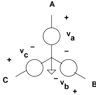
Figure 2: Three-Phase Voltage Source
