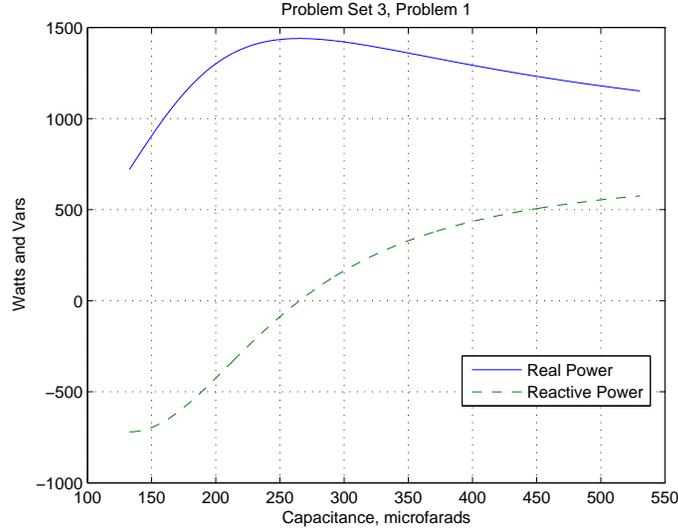
Figure 3: Real and Reactive Power Vs. Capacitor Value
