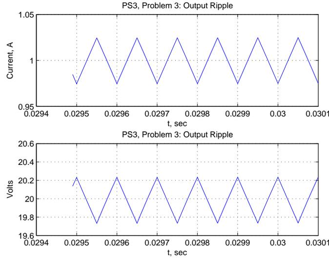
Figure 8: Ripple Current and Voltage for Boost Converter
