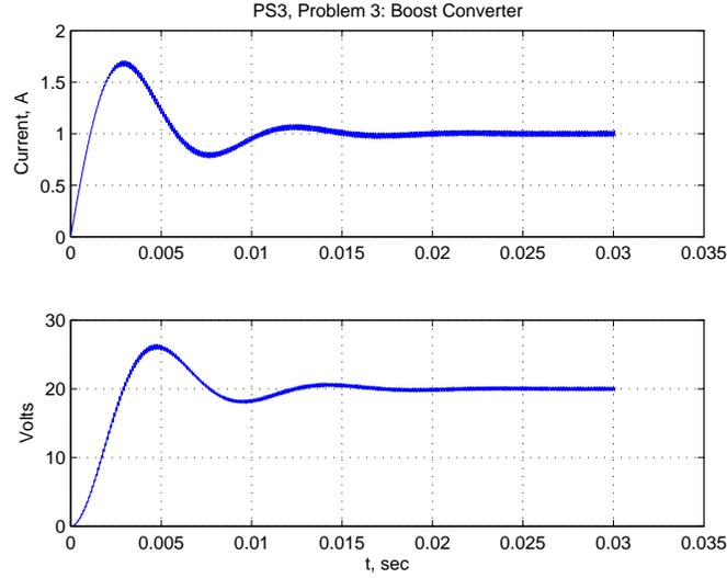
Figure 7: Buildup Transient for Boost Converter
