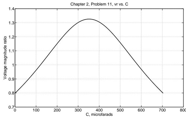
Figure 6: Voltage transfer ratio vs. Capacitance
