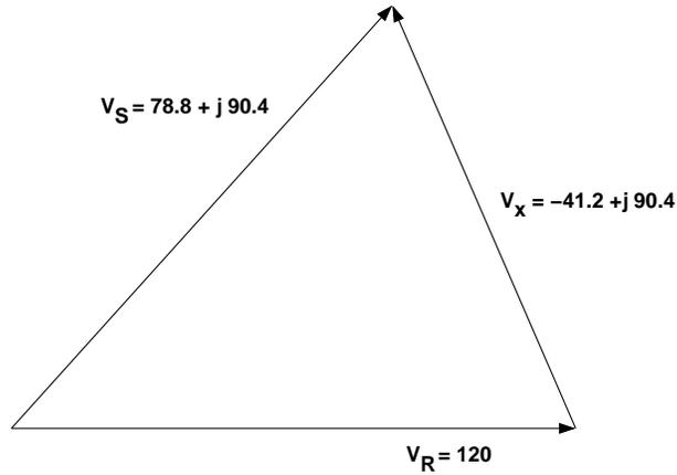
Figure 5: Phasor Diagram: compensated to equal voltage
