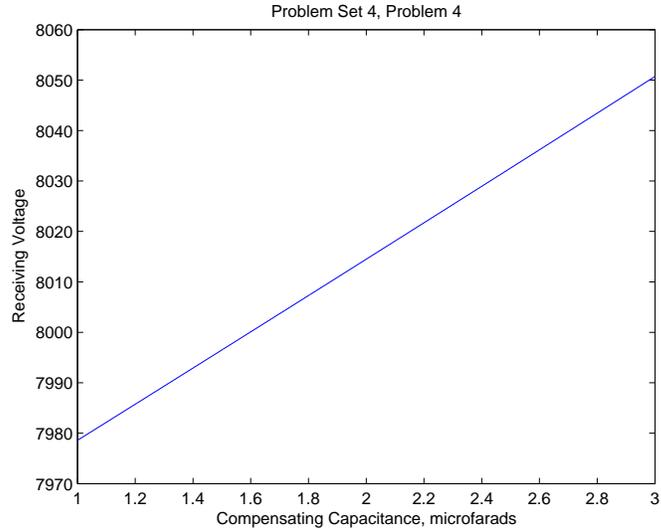
Figure 10: Receiving end voltage magnitude vs. compensating capacitor
