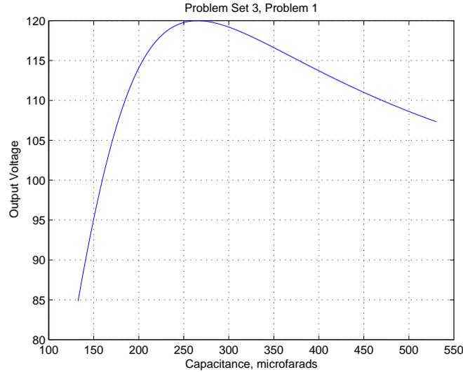
Figure 2: Voltage vs. Compensating Capacitor Value
