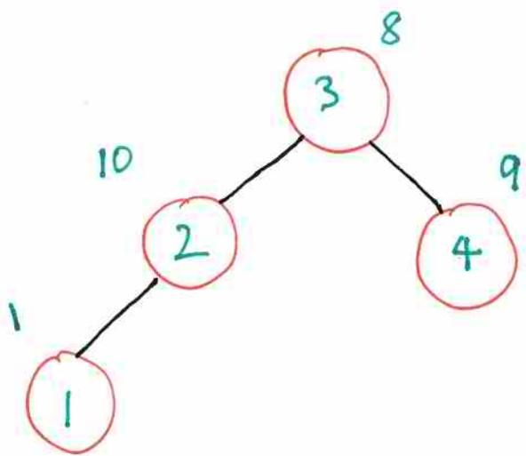
$$\begin{aligned} \text{cost} &= w_1 \times \text{depth}_1 + w_2 \times \text{depth}_2 \\ &+ w_3 \times \text{depth}_3 + w_4 \times \text{depth}_4 \\ &= 1 \times 3 + 10 \times 2 \\ &+ 8 \times 1 + 9 \times 2 \\ &= 49 \end{aligned}$$
