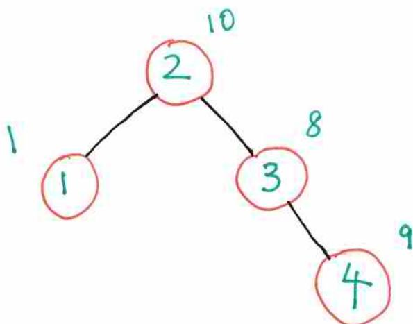
$$\begin{aligned} \text{cost} &= w_1 \times \text{depth}_1 + w_2 \times \text{depth}_2 \\ &+ w_3 \times \text{depth}_3 + w_4 \times \text{depth}_4 \\ &= 1 \times 2 + 10 \times 1 \\ &+ 8 \times 2 + 9 \times 3 \\ &= 55 \end{aligned}$$
