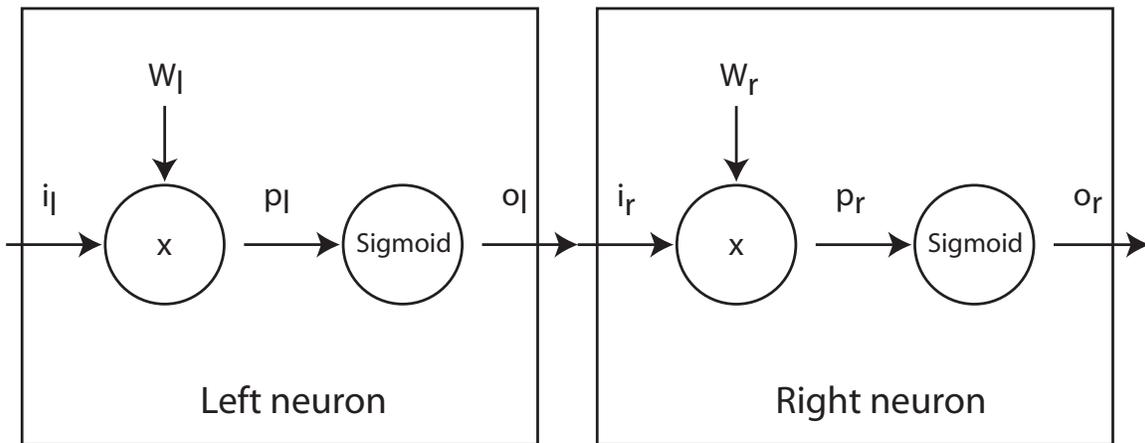
Note that the subscripts indicate layer. Thus,  $i_l$ ,  $w_l$ ,  $p_l$ , and  $o_l$  are the input, weight, product, and output associated with the neuron on the left while  $i_r$ ,  $w_r$ ,  $p_r$ , and  $o_r$  are the input, weight, product, and output associated with the neuron on the right. Of course,  $o_l = i_r$ .
